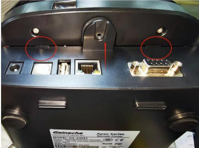
8. Card the bump of the stripper into the groove as shown below:
