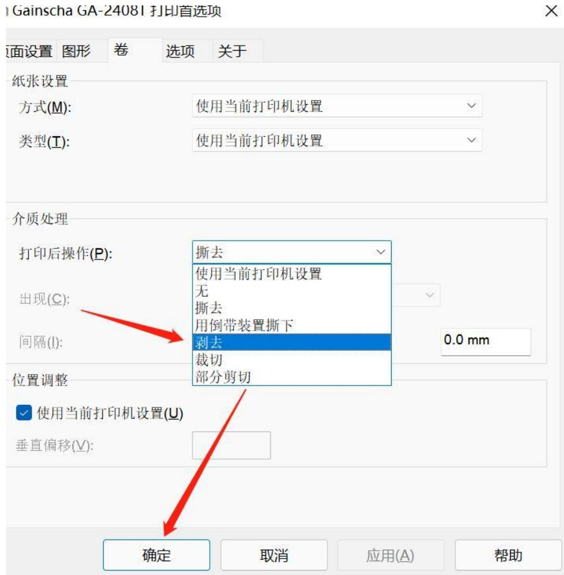
14. Check that the stripper is successfully installed. Open the BarTender for printing. See if the printer has a stripping action.
