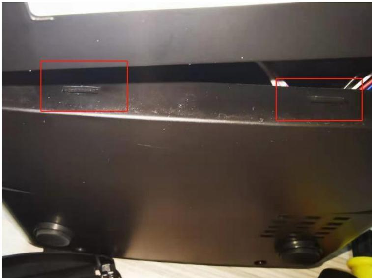
7. Hands hold the drawing circle in the picture, to the "arrow" direction of the rear bottom shell to hear a crisp sound after installing the bottom shell screw of the mouth on the figure below:
