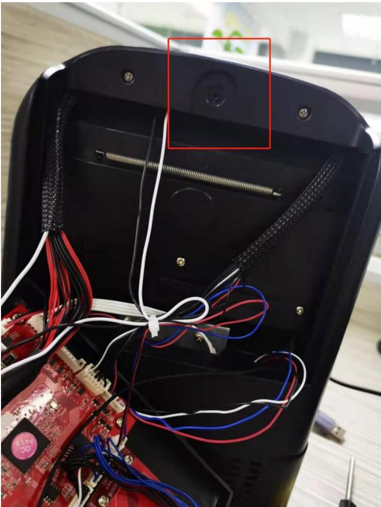
5. Find the wire connector for the stripper and insert the "Number 1 mark position" in the figure below
