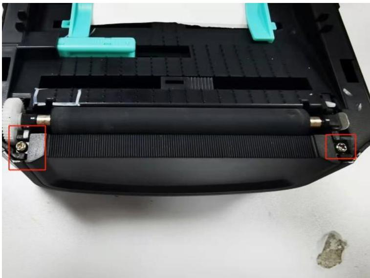
2. Lift the baffle up, and remove it:
