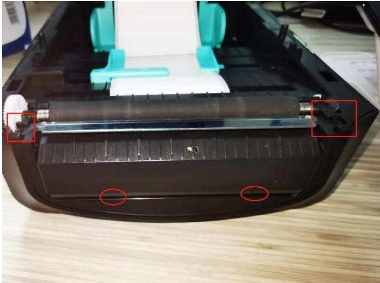
10. Open the stripper and pass the label bottom paper through the stripper as shown in the figure below:
