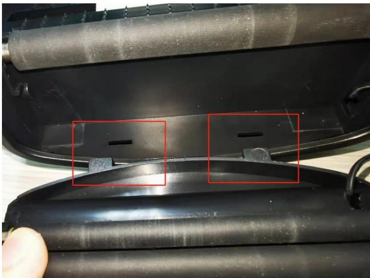
9. The screw hole of the stripper is stuck into the card slot, press the drawing circle in the picture inside, hear the "card" and install the stripper screw in the figure below:
